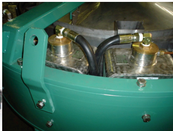
Figure 6. Two of the 16 coils making up the electromagnet of a vertical ring WHIMS unit capable of generating 1.0 T background intensity; note the oil outlets at the top of the coil box.
